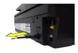
3. Disconnect the power cord from the ORIGINAL printer, and save it to use with the REPLACEMENT printer.
