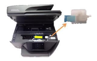
4. Lift at the slot on the left to open the printer. Remove the carriage restraint and save it to return the original printer.
