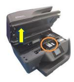
1. Turn the ORIGINAL printer on, lift the cover, and wait for the carriage to stop.
