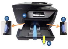
5. A: Lift up output tray.B: Pull out the Input tray.C: Press the handles and take out Input Tray.
