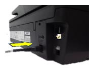
1. Connect power cord, using the power cord from original printer.
