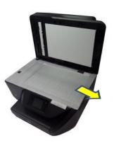
3. Open the scanner lid. Remove glass protective foam.
