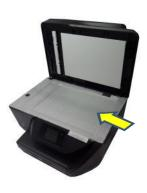
5. Open the scanner lid. Place the Glass Protector on top. Close the scanner lid.
