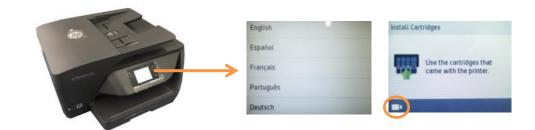
2. Press the Power button to turn on the replacement printer. Follow the instructions on the printer display.
